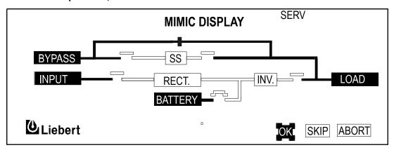
Press OK to close the SS contactors, turning on the Static Switch. Press SKIP only to proceed without closing the Static Switch contactors. Either selection brings up the screen enabling modification of input current limit.
